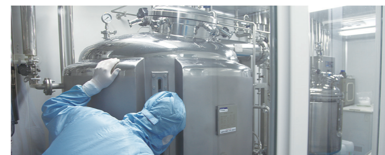
Fully automatic liquid dispensing system with the batch output of 1000 L
