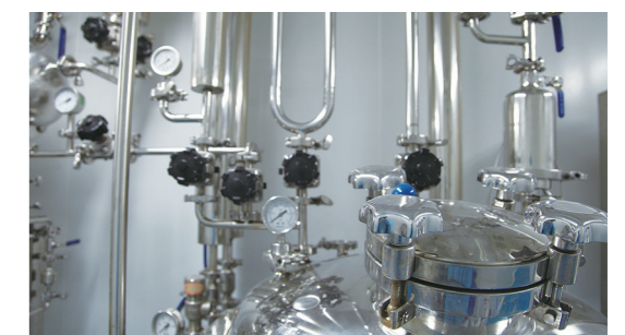
CIP&SIP, to ensure the sterility of the whole manufacturing process
